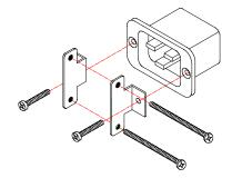
Figure 2. Retention Bracket assembly
